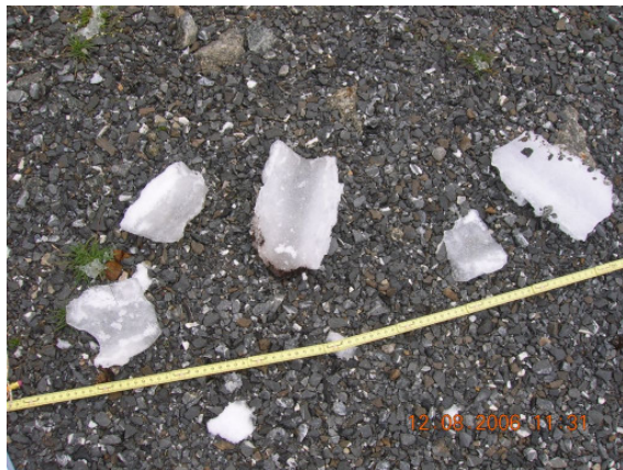
Fig. 5: Ice fragments from the E-40 wind turbine.
