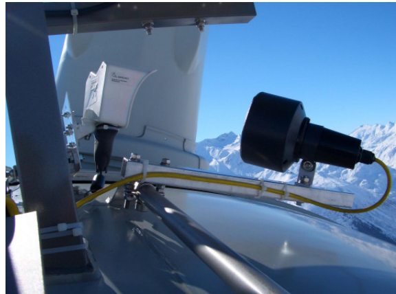
Fig. 3: Web cam mounted on the nacelle of the wind turbine. The lamp on the right is for heating purposes
