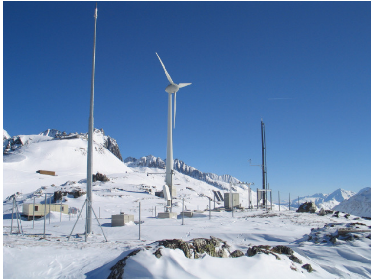
Figure 1: Alpine Test Site Guetsch. In the foreground, the meteorological test station can be seen, in the background the Enercon E-40 wind turbine.
