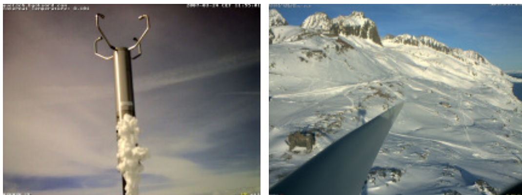
Left: image of Thies Ultrasonic anemometer on nacelle of the wind turbine. Right: image of rotor blade.
